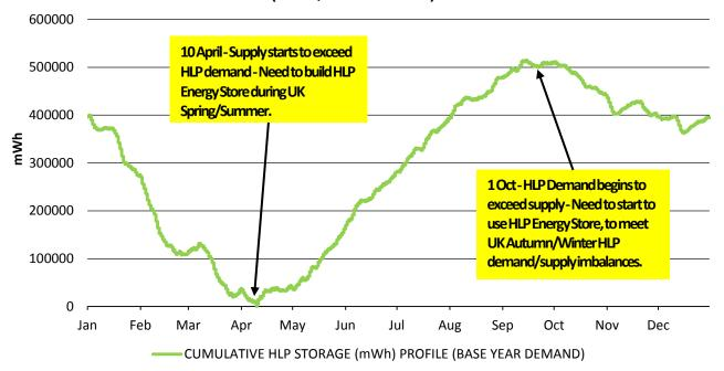
It was evident that the solar supply and heat, light, power demand created significant imbalance, so the simulator was run to provide a sensitivity analysis using reducing solar supply. It indicated that 60% of the storage requirement (above) came from the 25% of solar in the mix.
